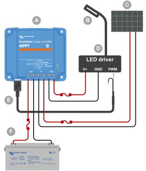
Wiring example - Controlling a streetlight LED driver.
