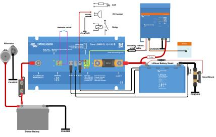
Application example with Phoenix VE.Bus Inverter rated at 3kVA and more
