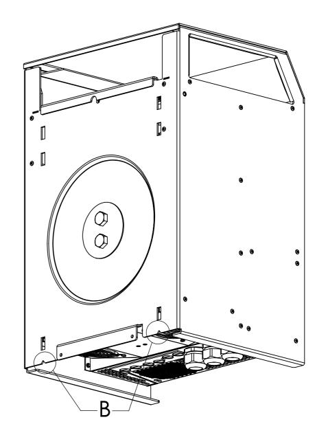
After mounting the MountingPlate to the wall Notice the bottom hooks extend more then the other hooks (A). Next notice the traingular cut-outs (B) at the back of the unit.
