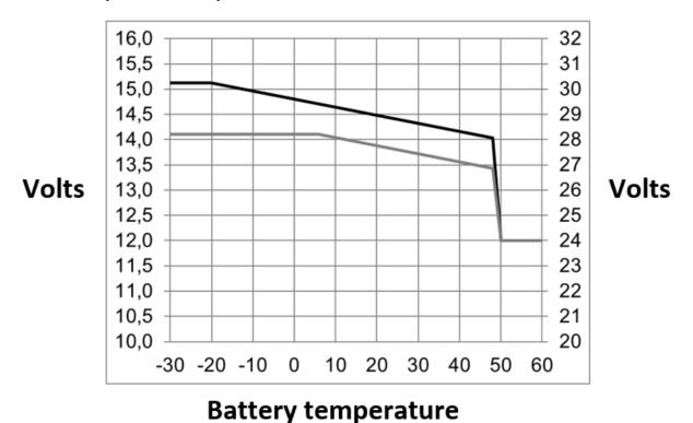
The above chart displays the default output voltages for Float and Absorption at 25 °C for 12 and 24V battery banks. For a 48V battery bank, multiply the 24V voltages by 2.
