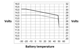
Default output voltages for Float and Absorption are at 25 °C for 12V or 24V battery bank, to arrive at 48V battery bank voltages, multiply the 24V voltages by a factor two.
