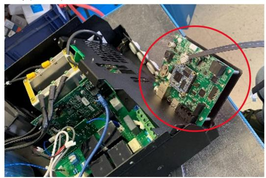
8 Insert the microSD card into the SD card slot with the contacts pointing upwards.
