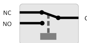
Relay configuration (not energised).
