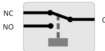
Internal operation of the programmable relay
