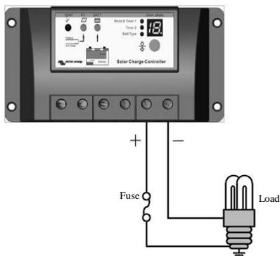
*Figure 3-3 Load Wiring*
