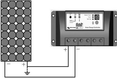
Figure 3-4 Solar wiring
