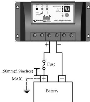
*Figure 3-2 Battery connecting*
