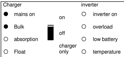
The AC input voltage is switched through and the charger operates in bulk mode.
