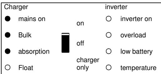
The mains voltage is switched through and the charger is on. The set absorption voltage, however, has not yet been reached. (BatterySafe mode)
