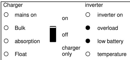
The inverter switched off due to excess ripple voltage on the battery terminals.
