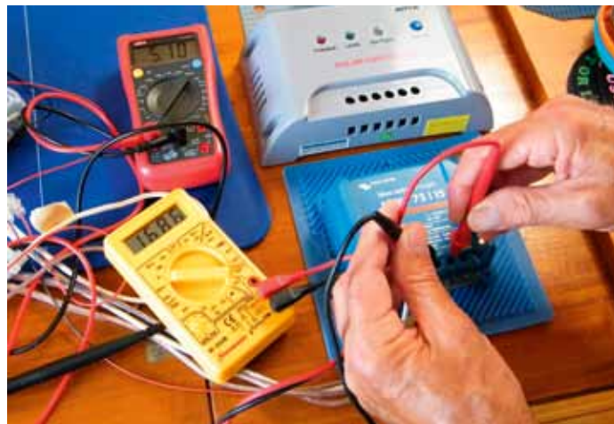
ABOVE All ready for testing. Nearest is the SunSaver 20, then MPPT30 and Victron 75/15. The data logger recorded power on the input of the regulator. BELOW The leads from the solar panel were fed through an ammeter to the unit under test. The voltage on both input and output was taken with a digital multimeter and the output current with a second digital multimeter. Readings were taken every five minutes
