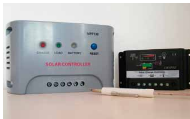
The MPPT30 Solar Controller on the left is available all over the internet but is best left there, in my opinion. I didn't even test the CMPT02 Solar Charge Controller on the right. It may be a useful regulator – internally it seemed better constructed than the MPPT30 – but the small size, lack of DC-DC converter components and lack of a microprocessor clearly indicated it was not an MPPT type
