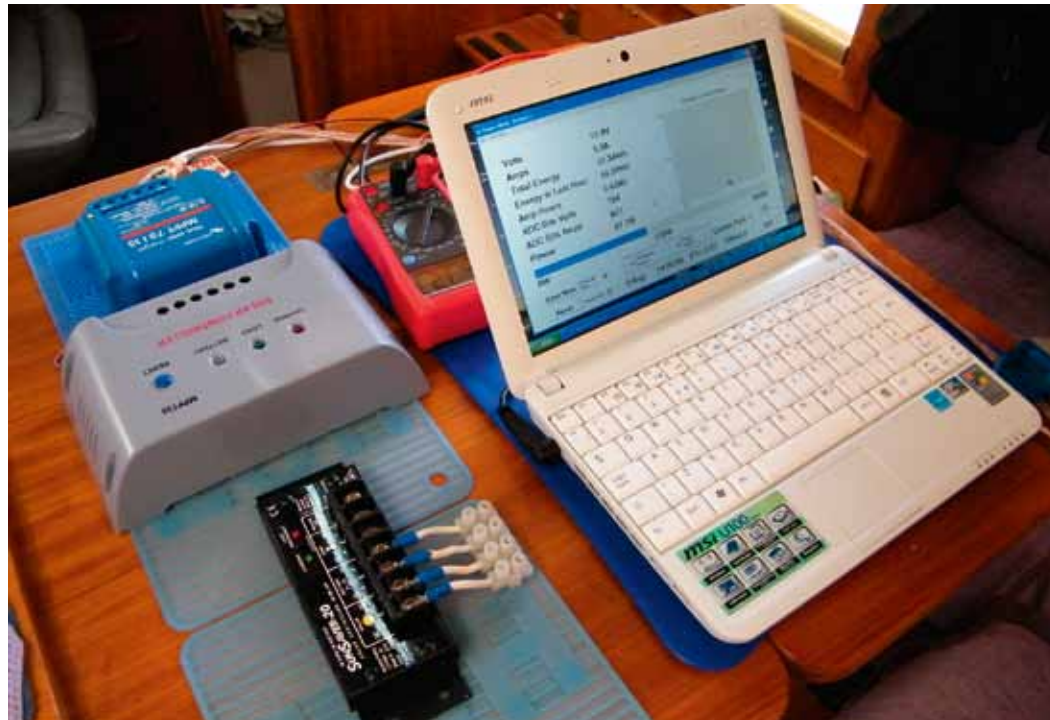
ABOVE All ready for testing. Nearest is the SunSaver 20, then MPPT30 and Victron 75/15. The data logger recorded power on the input of the regulator. BELOW The leads from the solar panel were fed through an ammeter to the unit under test. The voltage on both input and output was taken with a digital multimeter and the output current with a second digital multimeter. Readings were taken every five minutes
