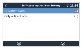
This setting allows ESS only to use battery power for essential loads. It also allows battery banks to be sized to get critical loads through the night without the battery being discharged into the non-essential loads.
