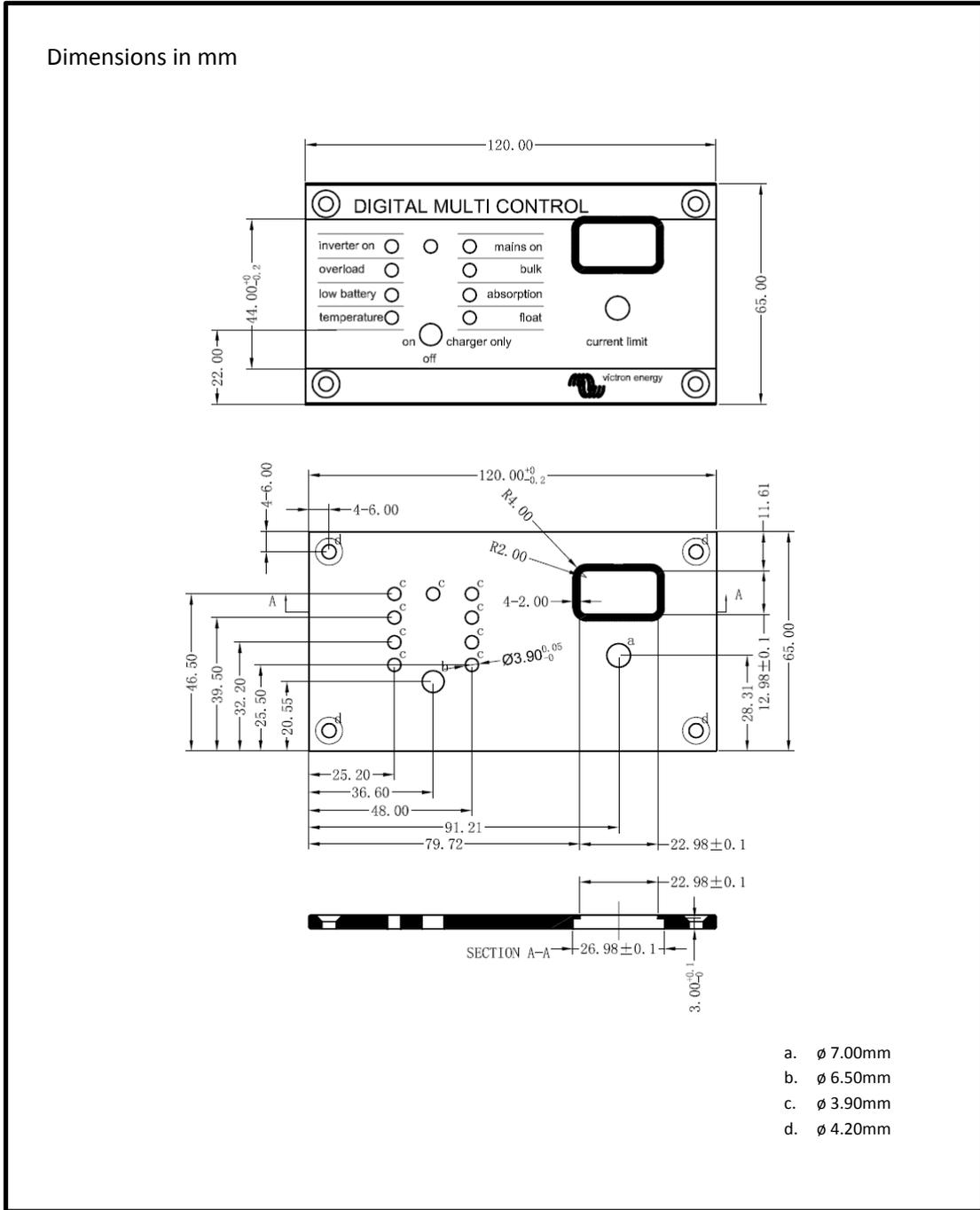
Dimensions of metal panel **REC020005000 Digital Multi Control 200/200A**
