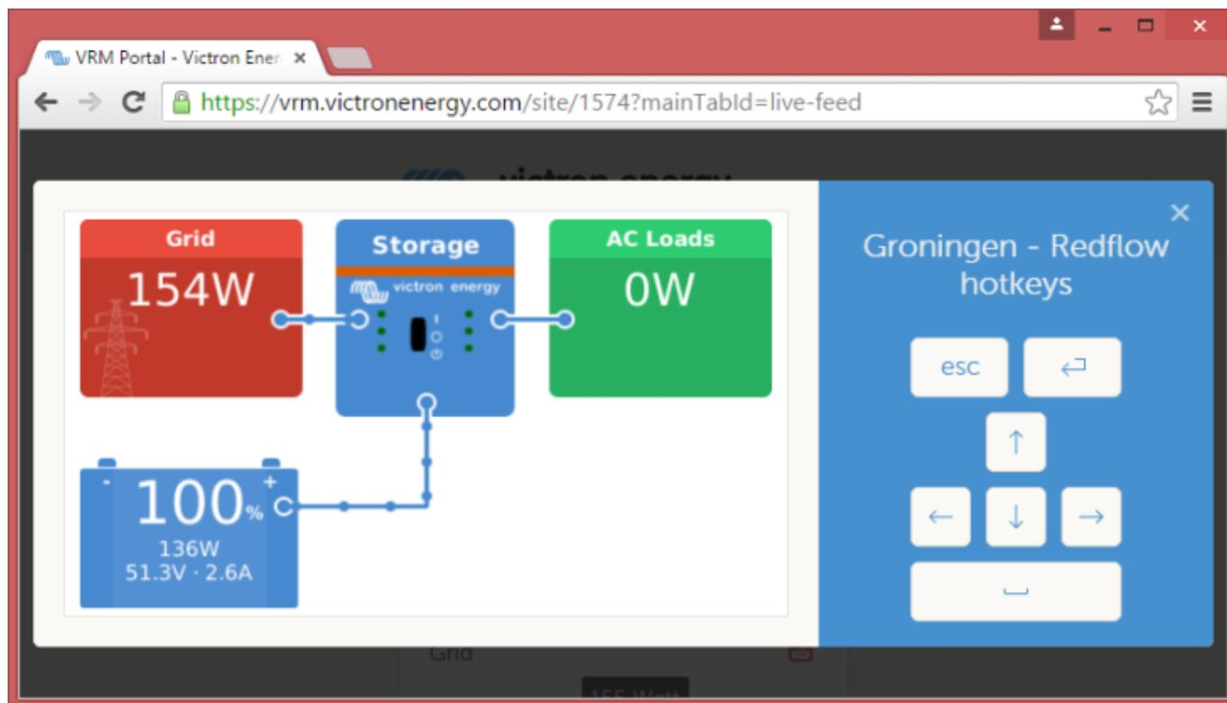
After enabling the feature in the CCGX setting menu, setting or disabling the password, and then restarting the CCGX, a new Menu Option will show on the VRM website. Click it to open the Remote Console.
