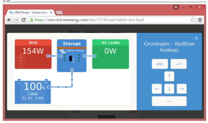
After enabling the feature in the CCGX setting menu, setting or disabling the password, and then restarting the CCGX, a new Menu Option will show on the VRM website. Click it to open the Remote Console.
