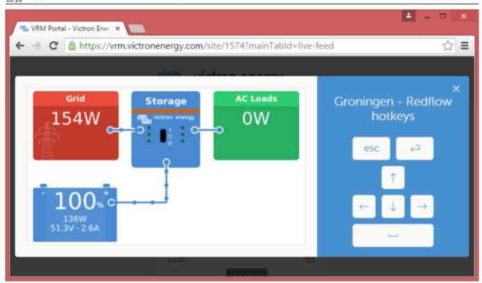
After enabling the feature in the CCGX setting menu, setting or disabling the password, and then restarting the CCGX, a green button will show on the VRM website. Click it to open the Remote Console.
