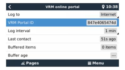
Check 'Last contact'. If this shows dashes or a time that is much larger than 'Log interval', the CCGX is not able to contact the VRM database.
