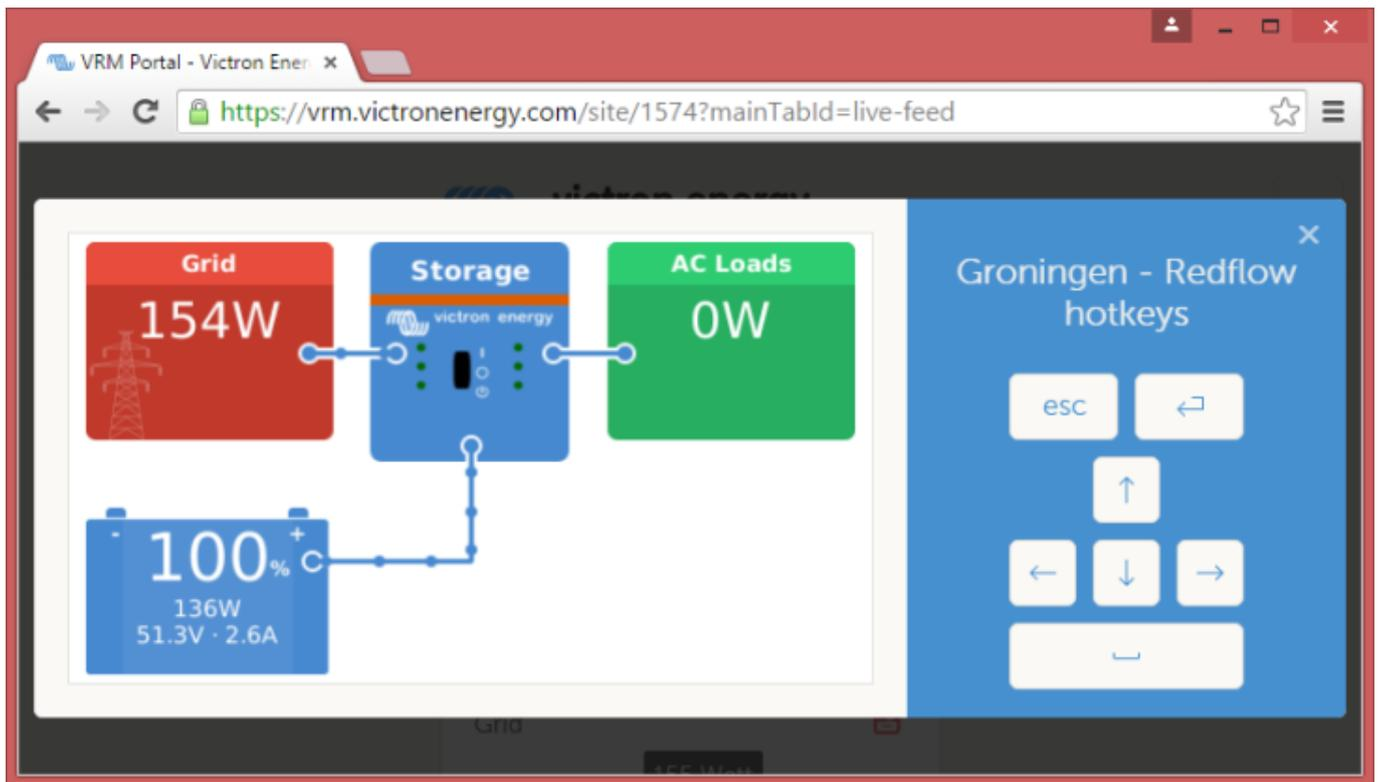
After enabling the feature in the CCGX setting menu, and then restarting the CCGX, a green button will show on the VRM website. Click it to open the Remote Console.
