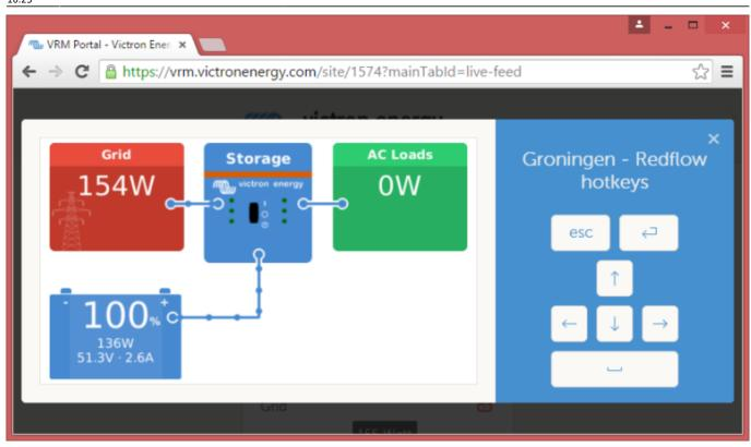
After enabling the feature in the CCGX setting menu, and then restarting the CCGX, a green button will show on the VRM website. Click it to open the Remote Console.
