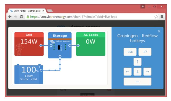
The Remote Console on VRM feature allows full remote control of a CCGX, over the internet:
