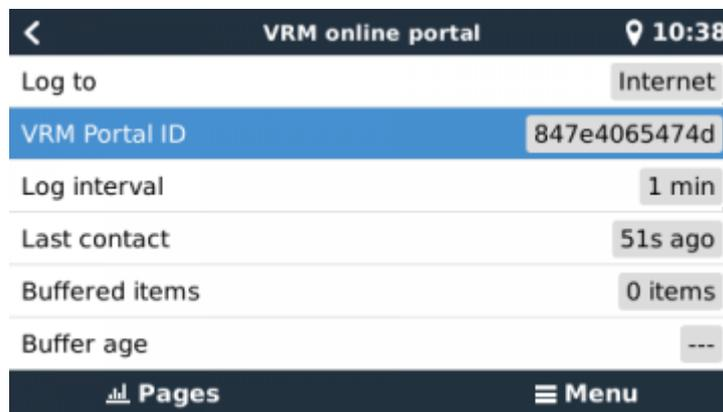
1) Check that 'Log To' is set to 'Internet'. If this is set to 'microSD or USB storage', then the CCGX will not log directly to the VRM portal using an internet connection, but will log to inserted microSD or USB storage. The database files on this storage should be uploaded manually on the VRM portal.
