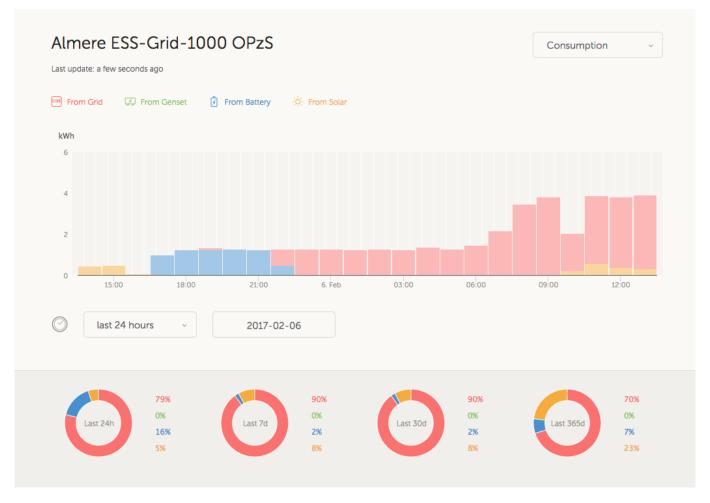
These graphs work on information calculated by the Color Control GX or Venus GX, based on energy counter values read from connected devices.
