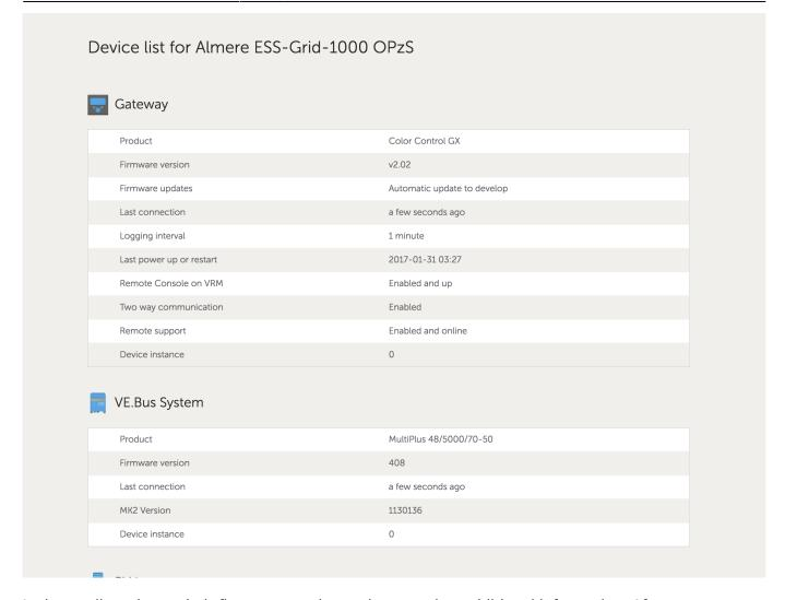
It shows all products, their firmware version and some other additional information. After disconnecting a product from the Venus-device or the Victron Global Remote, it is necessary to power cycle it (the CCGX, Venus GX or VGR). This will make the VRM Portal to empty the list and re-populate it based on the new information.
