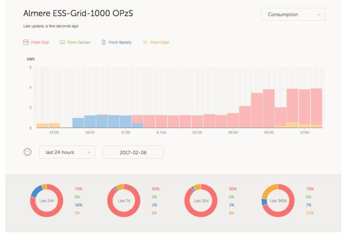
These graphs work on information calculated by the Color Control GX or Venus GX, based on energy counter values read from connected devices.
