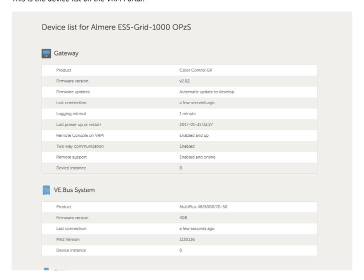
It shows all products, their firmware version and some other additional information. After disconnecting a product from the Color Control GX or the Victron Global Remote, it is necessary to power cycle it (the CCGX or VGR). This will make the VRM Portal to empty the list and re-populate it
