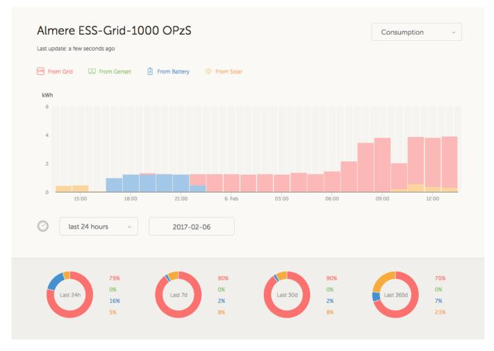
These graphs work on information calculated by the Color Control GX, based on energy counter values read from connected devices.
