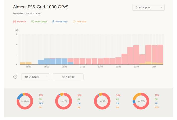
These graphs work on information calculated by the Color Control GX, based on energy counter values read from connected devices.
