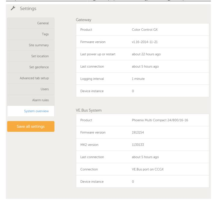
It shows all products, their firmware version and some other additional information. After disconnecting a product from the Color Control GX or the Victron Global Remote, it is necessary to power cycle it (the CCGX or VGR). This will make the VRM Portal to empty the list and re-populate it based on the new information.
