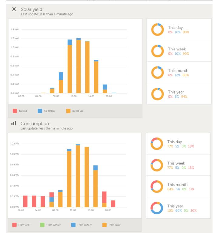
These graphs work on information calculated by the Color Control GX, based on energy counter values read from connected devices.
