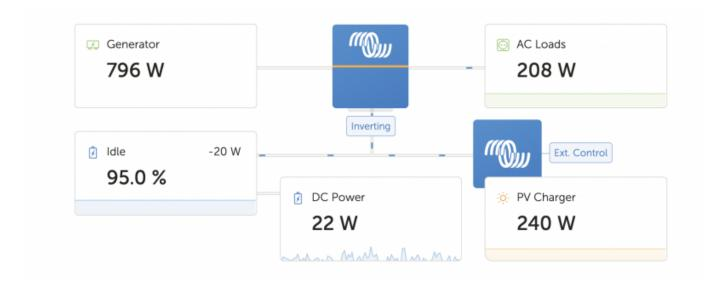
The information shown adapts itself to the system installed. For systems without an inverter/charger, separate blocks of information are shown, without connected lines and 'moving ants'.
