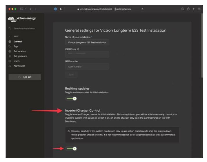
It is ONLY recommended to enable this easy system shutdown control for small systems in non-critical environments. It is STRONGLY recommended to leave this feature disabled for large mission critical systems, or where there are multiple users with access to the Admin controls.
