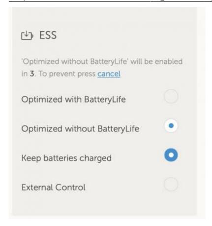
You will also be able to adjust the minimum state of charge. Note that setting the minimum state of charge will not be possible when the ESS is set to 'keep batteries charged' as that mode will override and charge the battery to 100% when possible.
