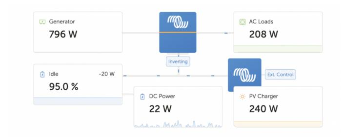
The information shown adapts itself to the system installed. For systems without an inverter/charger, separate blocks of information are shown, without connected lines and 'moving ants'.
