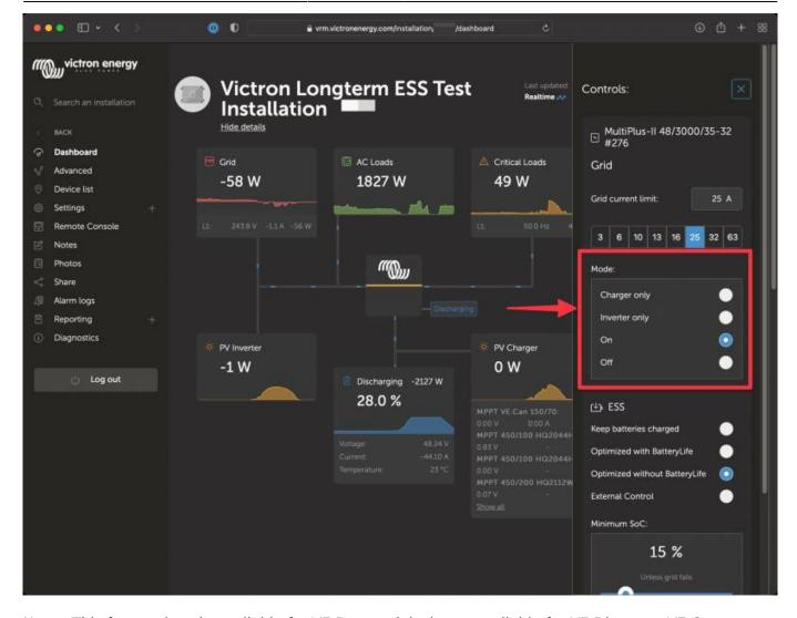
Note - This feature is only available for VE.Bus models, is not available for VE.Direct, or VE.Can inverters. Also, there is a limitation where these controls are not available when using a Digital Multi Control, or VE.Bus BMS v1 in the system.
