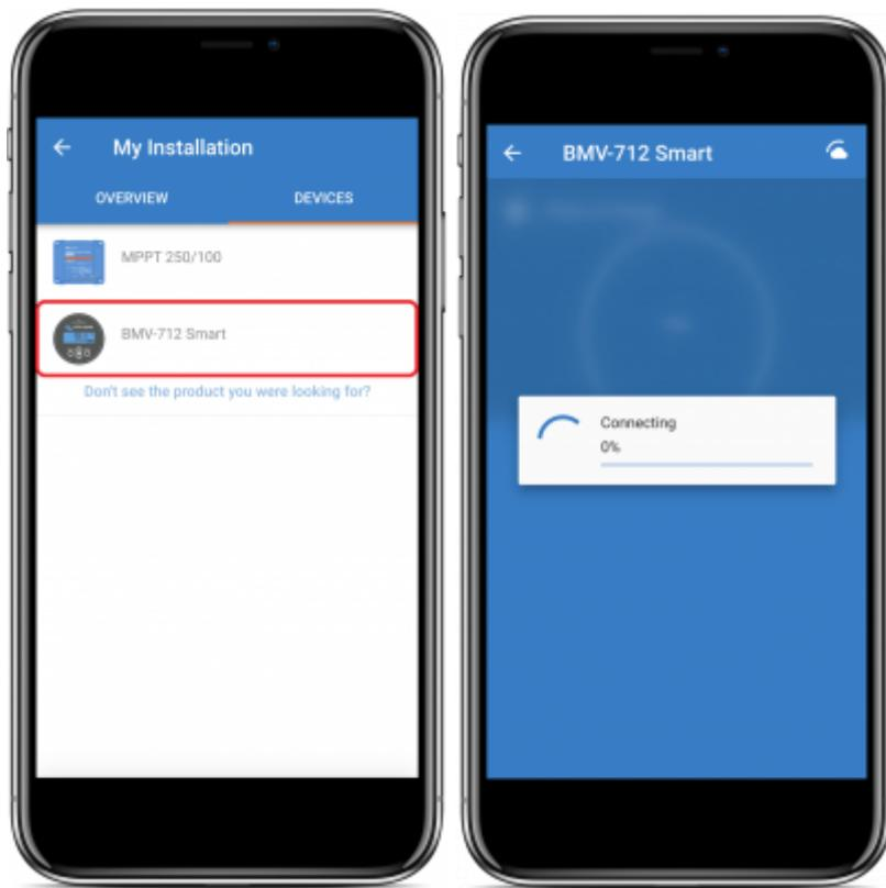
Immediately after initial connection settings and historical data will be downloaded, during this time a cloud symbol will remain in the upper right corner (this typically takes less than 30 seconds).
