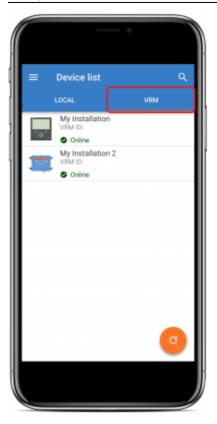
When a VRM installation is selected it will take a few seconds for a connection to be made, once the connection is established two tabs will appear, an 'OVERVIEW' tab and a 'DEVICES' tab.
