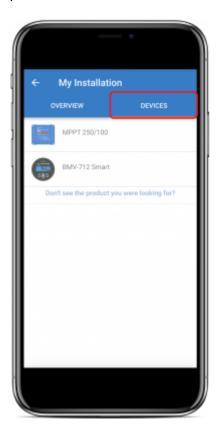
If using a tablet or PC, the 'DEVICES' tab is shown as a panel on the right side of the same screen.
