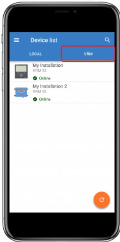
When a VRM installation is selected it will take a few seconds for a connection to be made, once the connection is established two tabs will appear, an 'OVERVIEW' tab and a 'DEVICES' tab.
