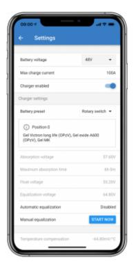
For small MPPT Solar Charger models there is only one preset. Larger models feature a rotary switch, the battery page shows the setting of the rotary switch.
