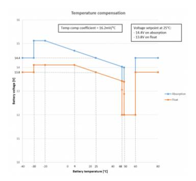
With a Smart Battery Sense is installed; the actual battery temperature will be used for compensation; throughout the day.
