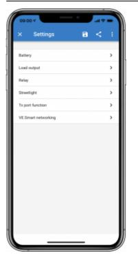
The settings page is accessed by clicking on the Cog icon at the top right of the Home page. The settings page provides access to view or change the settings of the Battery; Load; Streetlight; and Port functions. From this page you can also view Product information such as the Firmware versions installed on the MPPT Solar Charger.
