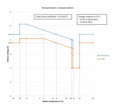
With a Smart Battery Sense is installed; the actual battery temperature will be used for compensation; throughout the day.
