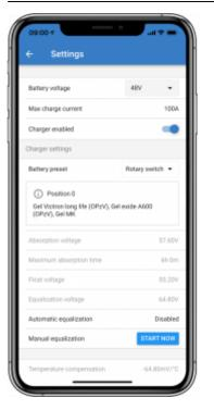
For small MPPT Solar Charger models there is only one preset. Larger models feature a rotary switch, the battery page shows the setting of the rotary switch.
