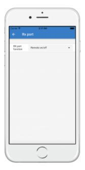
The Rx pin on the VE.Direct connector can be used for other functions. This functionality was introduced in firmware version 1.17. Available options:
