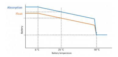
With a Smart Battery Sense is installed; the actual battery temperature will be used for compensation; throughout the day.
