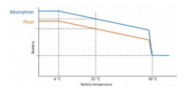
With a Smart Battery Sense is installed; the actual battery temperature will be used for compensation; throughout the day.
