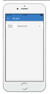
The Rx pin on the VE.Direct connector can be used for other functions. This functionality was introduced in firmware version 1.17 and applies to the 10A, 15A and 20A chargers with a load output. Available options:
