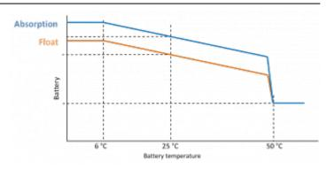
With a Smart Battery Sense is installed; the actual battery temperature will be used for compensation; throughout the day.
