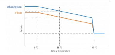
Note that the temperature compensation is not dynamic during operation. The charger uses its internal temperature for battery temperature compensation when the charger has been idle for at least one hour, i.e. when the charger is not actively charging a battery or supplying a load.
