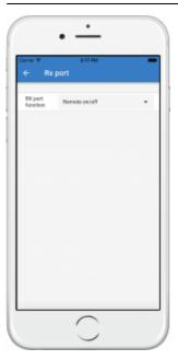
The Rx pin on the VE.Direct connector can be used for other functions. This functionality was introduced in firmware version 1.17 and applies to the 10A, 15A and 20A chargers with a load output. Available options:
