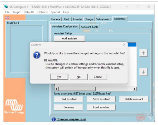
Now upload the converted file. On the VRM Portal, go to the Device List  $\rightarrow$  Remote VEConfigure menu  $\rightarrow$  'Upload' the converted file.
