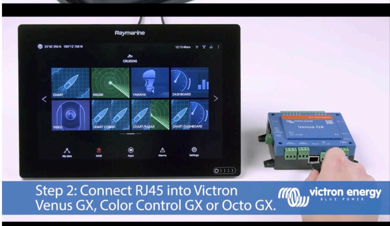
Step 2: Connect RJ45 into Victron
