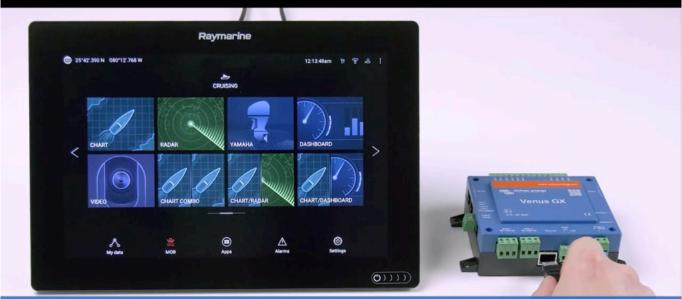
Step 2: Connect RJ45 into Victron
