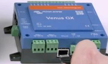
Step 2: Connect RJ45 into Victron Venus GX, Color Control GX or Octo GX.
