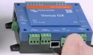
Step 2: Connect RJ45 into Victron Venus GX, Color Control GX or Octo GX.
