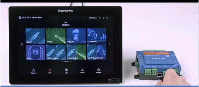
Step 2: Connect RJ45 into Victron
