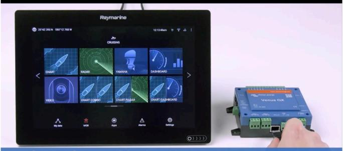
Step 2: Connect RJ45 into Victron
