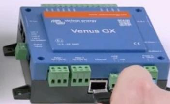
Step 2: Connect RJ45 into Victron Venus GX, Color Control GX or Octo GX.
