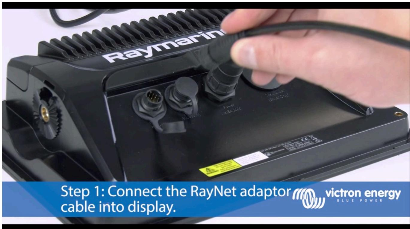
Step 1: Connect the RayNet adaptor
