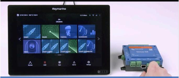
Step 2: Connect RJ45 into Victron
