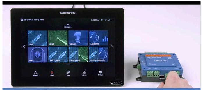
Step 2: Connect RJ45 into Victron
