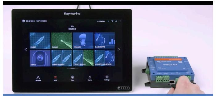
Step 2: Connect RJ45 into Victron
