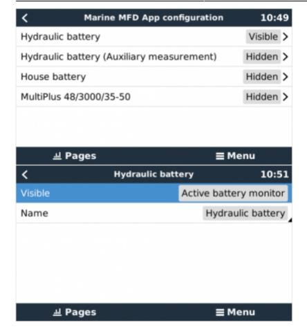
No other settings, such as IP addresses or similar are required. The GX device and the Navico devices connect to each other using a technology called linklocal addressing.
